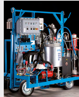
WIWA DUOMIX 333 PFP ATEX, for intumescent fire protection material
