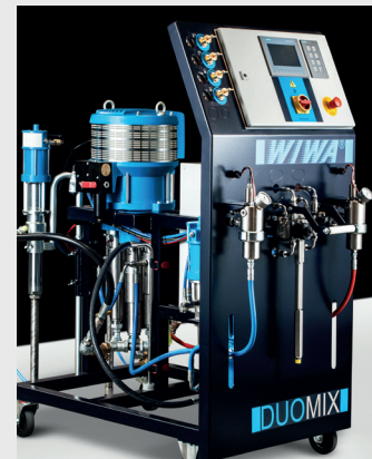
WIWA DUOMIX, pneumatic plural component spray equipment
